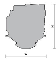
L = 1236 mm ₩ = 780 mm H = 793 mm Dry weight (without marine gear) = 605 kg
